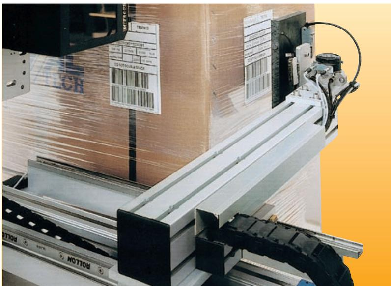
scanner which also detects the presence of the label on the pallet, and will initiate a second cycle to compensate if necessary, or a signal to stop the production line.
