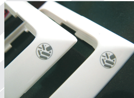
Laser marking on polyamide
