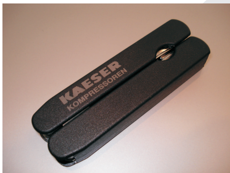
Laser marking on painted steel
