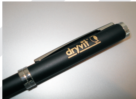
Laser marking on painted metal
