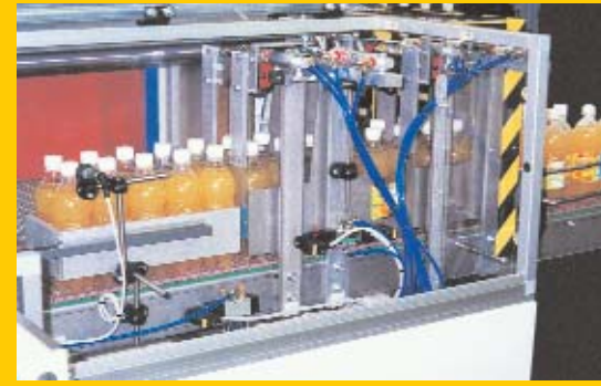
Quick feeding with partition on two rows. Output up to 15 packages minute. Sizes: 3x2, 4x2, 5x2.
